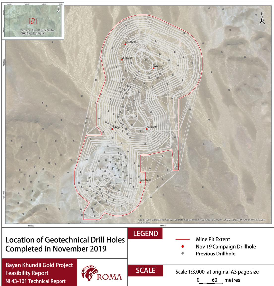
Figure 16-7 Location of Geotechnical Drill Holes Completed in November 2019.
