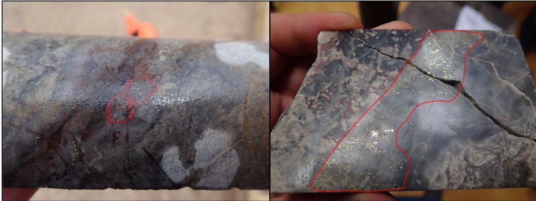
Figure 7-7 Visible gold in Bayan Khundii quartz veins, circled in red. (Tetra Tech, 2019a)
