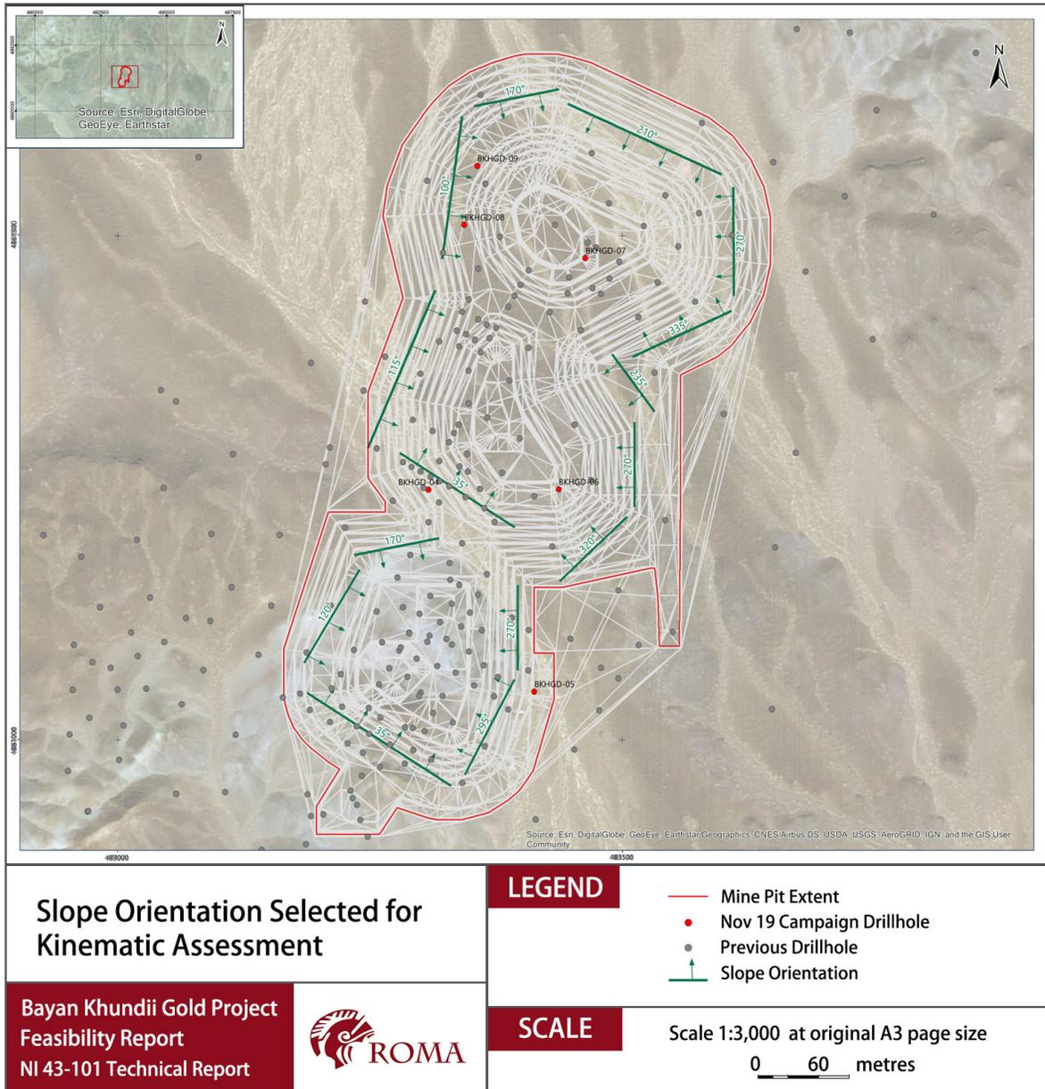
Figure 16-8 Slope Orientation Selected for Kinematic Assessment.
