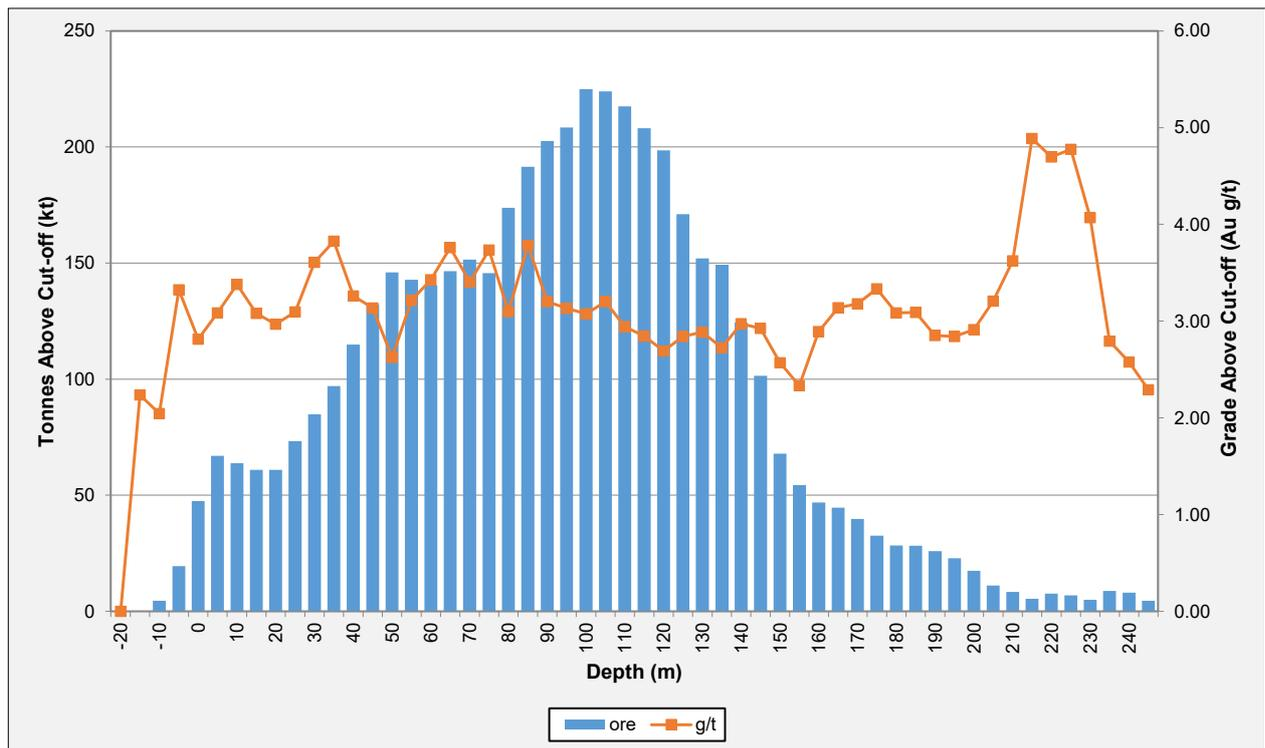
Figure 16-6 Altan Nar - Tonnes and Grades by Depth
