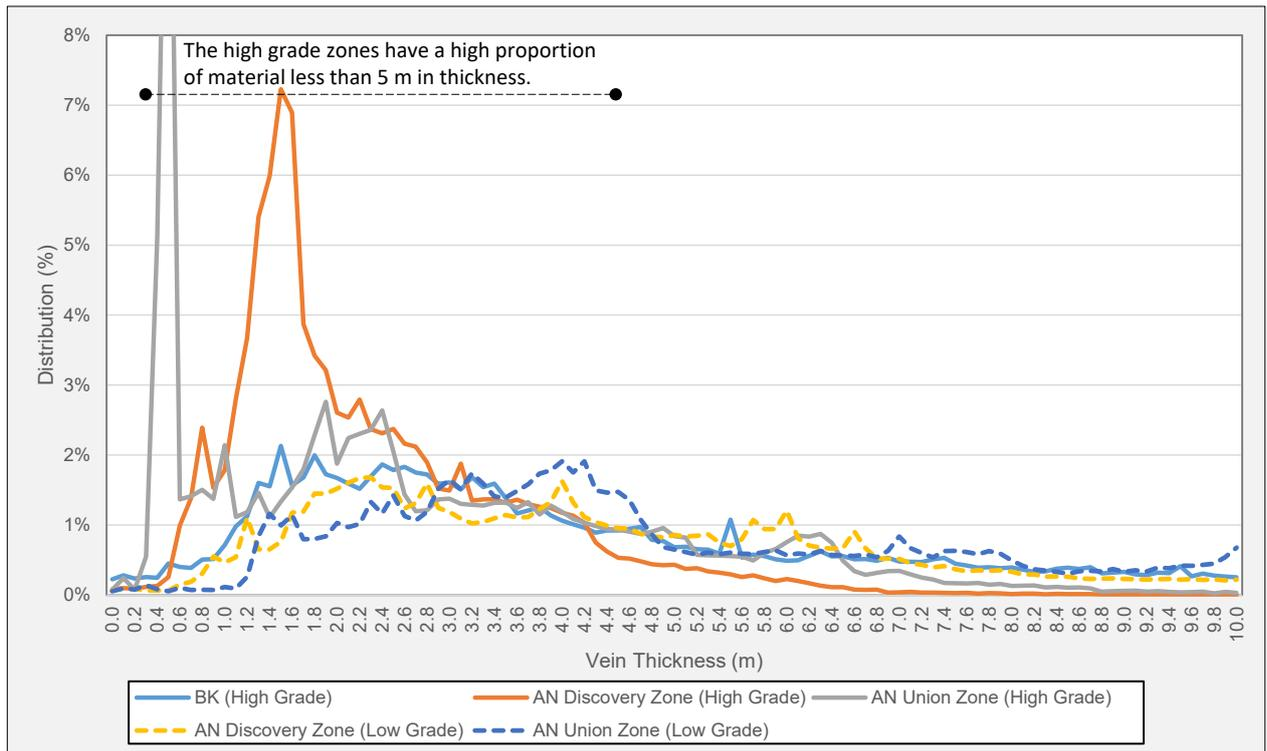
**Figure 16-2 Vein Thickness Cumulative Distribution**
