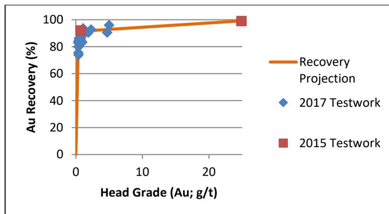
**Figure 13-8 Bayan Khundii Feed Grade-Recovery Relationship (0-6 g/t Au)**
