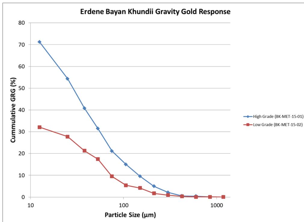
**Figure 25** - Bayan Khundii metallurgical sample gravity-gold-recovery size fraction recovery graph
